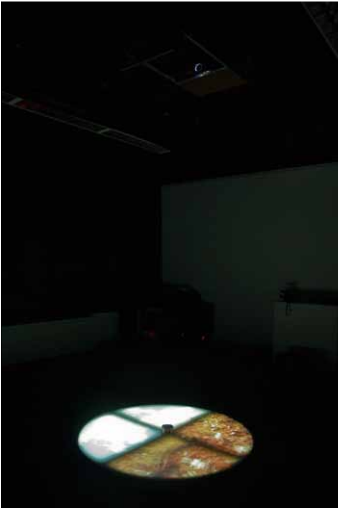
In the Cycles installation viewers enter a darkened space. As they enter the space an infrared sensor monitors their movement and activates the piece. A video projector is ceiling mounted and projects a circular image on the exhibition floor. Four-channel surround sound is monitored through speakers positioned in the four corners of the space to create an enveloping and drifting aural experience. In the installation viewers are encouraged to walk around the projection and intersect four laser beams. As viewers move around the circular pool of light they trip the laser sensors and the software loads four movies, randomly picked from a database of files. If multiple viewers occupy the space multiple videos run simultaneously to create an
